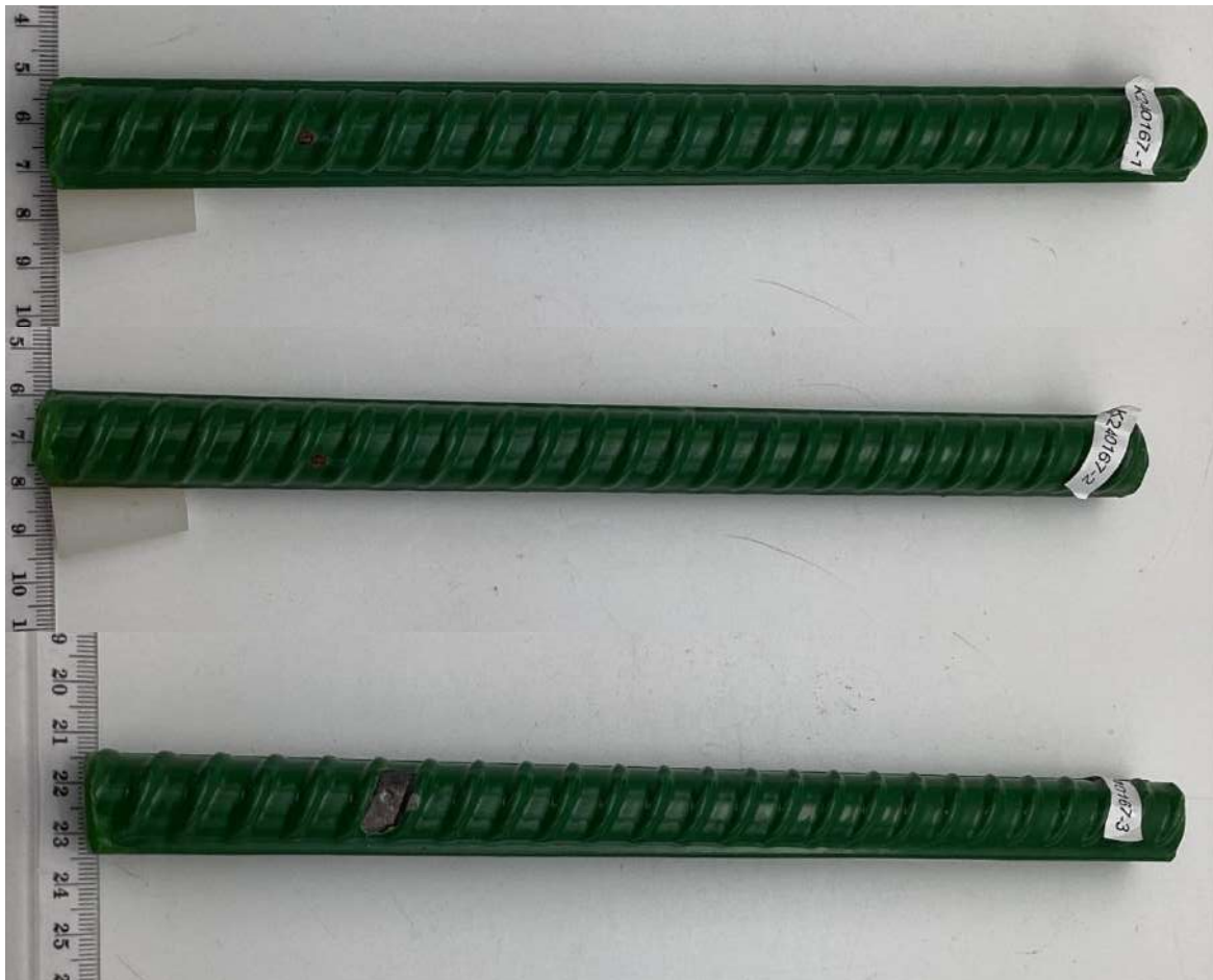
Complete sample after Cathodic disbondment
