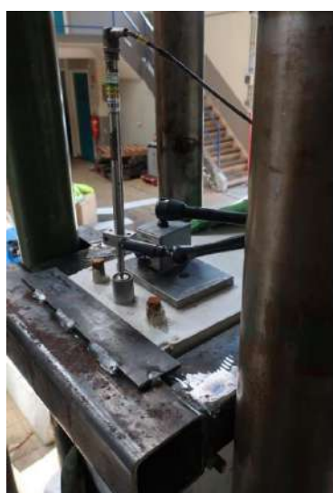
Attachment LVDT topside
