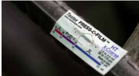
Surface Profile of Abrasive Blast - Cleaned Steel Using a Replica Tape
