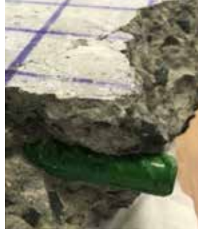
Fig 9. After Breaking Concrete Block with ECR
