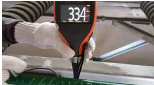
Coating Thickness Measurement
