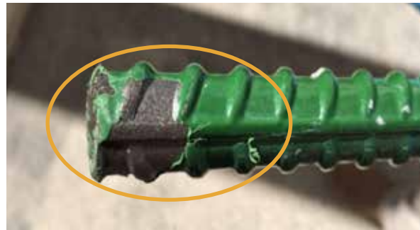
Fig 12. No Sign of Corrosion Underneath the Epoxy Coating
