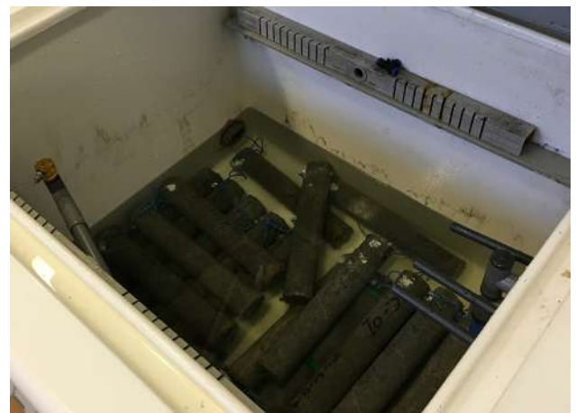
Fig. 2. The samples immersed in 15% NaCl - solution during wetting cycle of Southern Exposure test.
