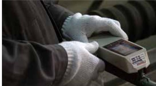
*Coating Thickness Measurement*
