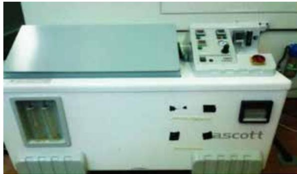
Fig 1. Salt Spray Chamber
